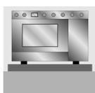
SI L'APPAREIL EST PLACÉ SUR UN SUPPORT, IL DOIT ÊTRE INSTALLÉ DE FAÇON À CE QU'IL NE GLISSE PAS DE CE SUPPORT.
